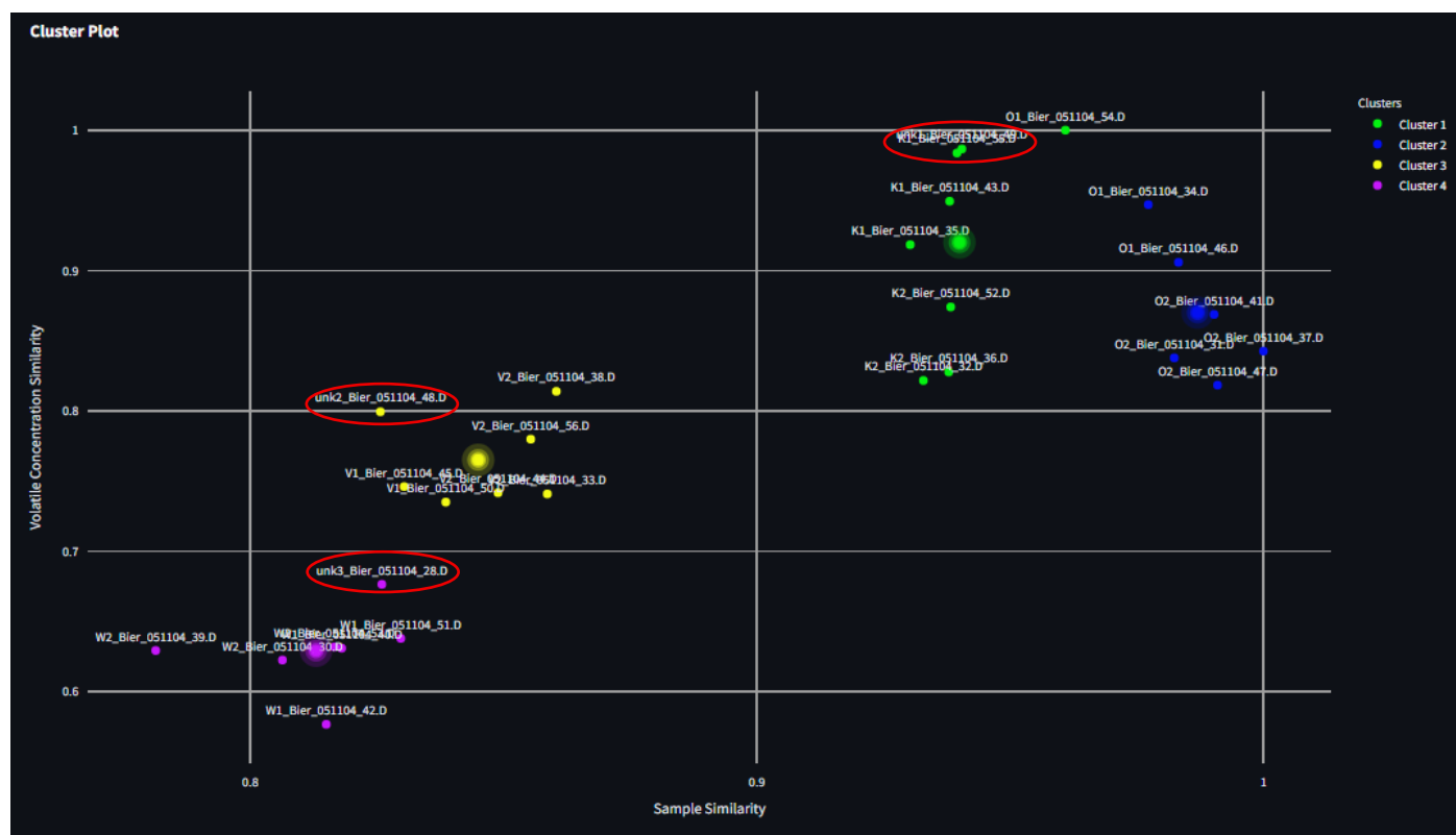
Figure 6: Unknown challenge samples projected into cluster feature space – the previously unknown samples are encircled in red.
